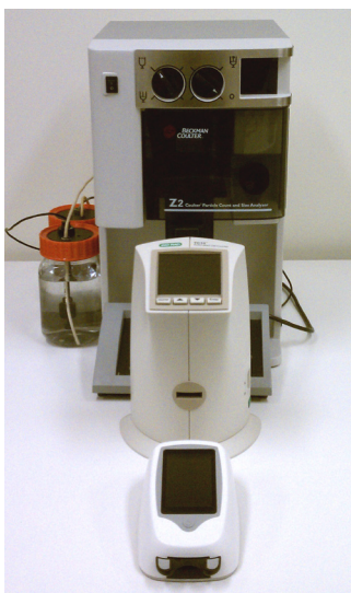
Fig. 1 – Photograph of the three systems evaluated in this application note. Juxtaposition of the systems highlights the relative size of each and the small footprint of the Moxi Z. From back to front: Beckman Coulter Z2, BioRad TC10, Orflo Moxi Z.
