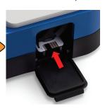
5) Pipette 60uL of Stained Sample Into the Cassette. Close Door. Test Begins.
