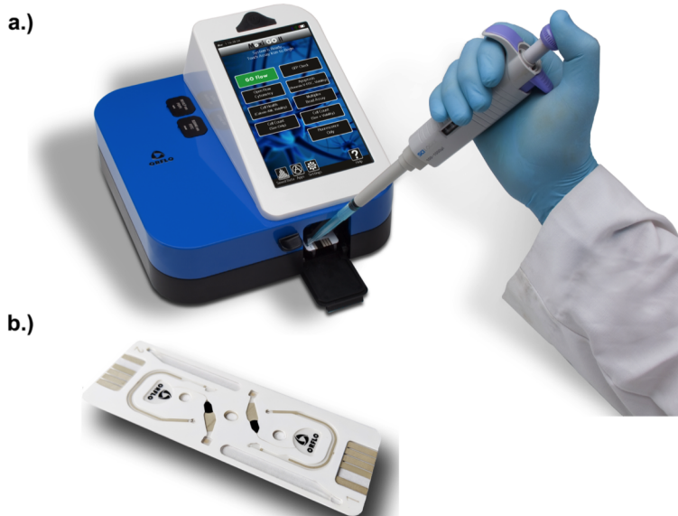
Figure 1 – a.) Orflo's Moxi GO II – Cell Health Analyzer. Image shows user loading a sample into the two-test disposable flow cell. The Moxi GO II is a flow cytometer/cell health analyzer with a 488nm laser and two fluorescence recording channels (2 PMT's with emission filters at 525/45nm filter and a user-swappable 561nm/LP or 646nm/LP). b.) Two-test, disposable flow cell "cassette"
